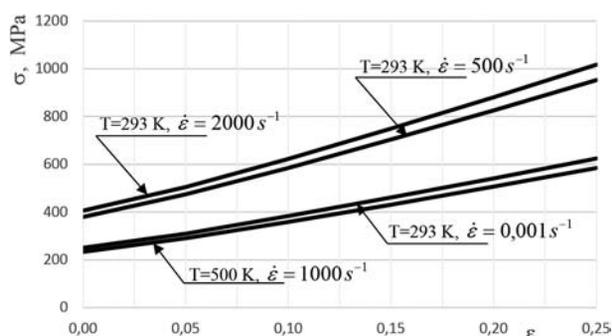
Figure 5 — Predicted stress-strain curves in 15G2ANb steel using the Johnson–Cook equation (5)
