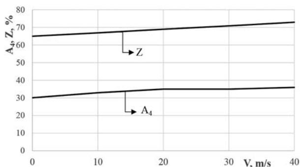
Figure 4 — Plasticity parameters of steel 15G2ANb:  $Z$  — reduction of area at fracture;  $A_4$  — strain for various stretching speed
