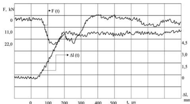
Figure 3 — The dependence force on the time  $F(t)$  and displacement  $\Delta l(t)$  for a dynamic steel tensile test 15G2ANb on a rotary hammer for the stretching speed  $V_n = 40 \text{ ms}^{-1}$  [10]
