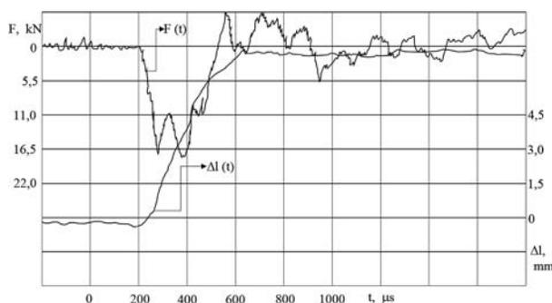
Figure 2 — The dependence force on the time  $F(t)$  and displacement  $\Delta l(t)$  for a dynamic steel tensile test 15G2ANb on a rotary hammer for the stretching speed  $V_n = 30 \text{ ms}^{-1}$  [10]
