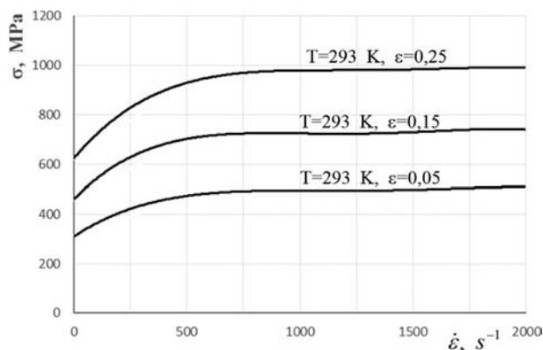
Figure 6 — Stress-strain rate curves in 15G2ANb steel for different strain values
