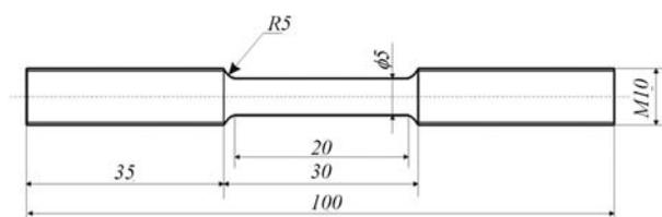
Figure 1 — The geometry of the sample for static and dynamic stretching tests
