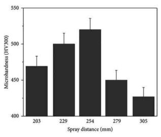
Figure 3 — Microhardness Co32Ni21Cr8Al0.5Y coating to different spray distances employed
