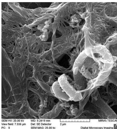
Figure 3 — Microstructure of heterogeneous DP of the complex lithium greases containing additives of ultradispersed particles of expanded graphite ( a ), diamond-graphite charge ( b ), carbon nanotubes ( c )
